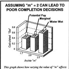
This graph shows how varying the value of "m" affects calculated water saturation when all else remains constant. A more accurate "m" is quickly and inexpensively estimated from visual rock analysis. This greatly increases your chances for success.
